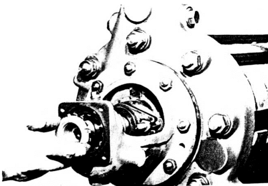
Fig. 81 - Mounting the inner race of the cylindrical roller bearing with clamping sleeve
