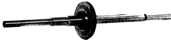
Fig. 70 - Shaft with first stage impeller
