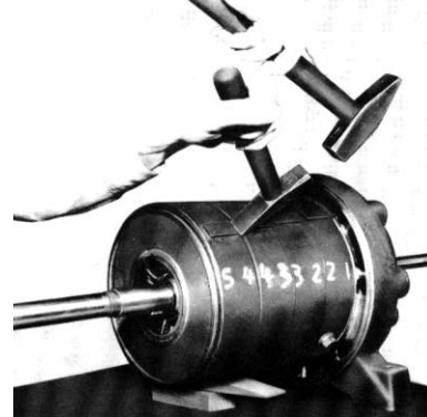
Fig. 62 - Slackening and removing the stage casing
