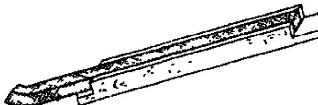
Fig. 19 – Slanted cut of the gasket
