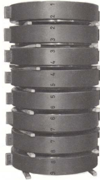
Figure 29 – Stacking the stage casings
